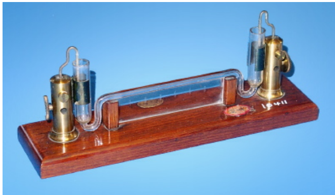
Lippman mercury galvanometer
